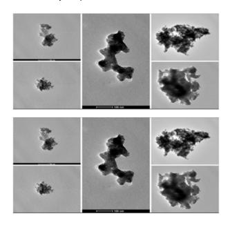
The tests show that for the nano-silica, by performing the following analysis, we can observe that the particle size obtained by this methodology is 8.04 nm, which is close to the range typically considered for nano-silica particles, which usually fall between 1 and 100 nm. On the other hand, for the ashes, the particle size obtained by this methodology is 143.816 nm, which is outside the range considered for nano particles.
