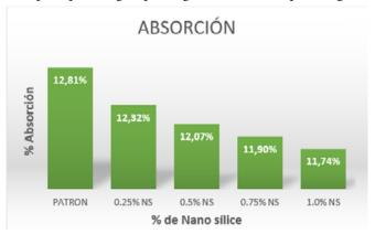
The graph shows the relationship between the absorption percentage and the nanosilica content (% NS). It is observed that as the concentration of nanosilica increases, the absorption percentage progressively decreases. The highest absorption value (12.81%) is found in the reference sample (PATRÓN), while the lowest value (11.74%) corresponds to the sample with 1.0% nanosilica. This indicates that the incorporation of nanosilica reduces the absorption of the material.
