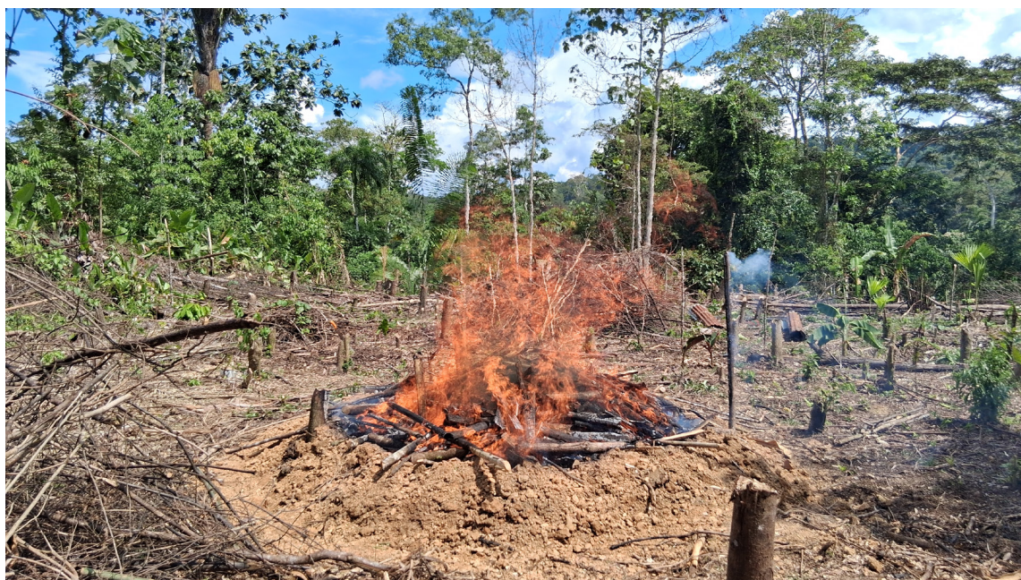
Figure 4. Pyrolysis in a flame curtain kiln.
