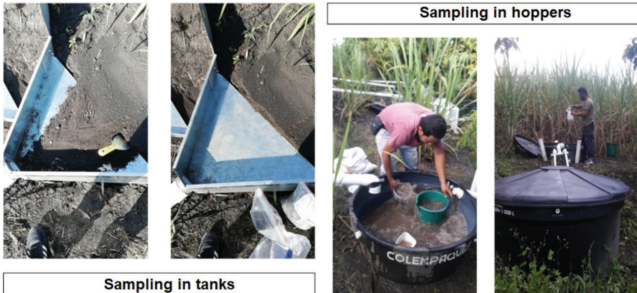
Figure 2. Sampling in the hoppers and tanks of the runoff plots in the department of Santander (municipality of Vélez).
