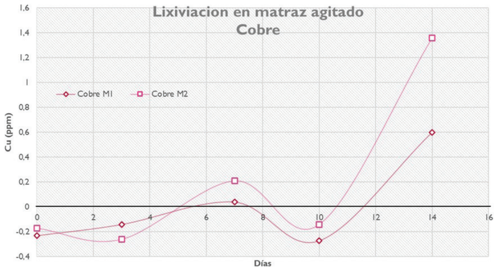
Figure 4. Changes in dissolved copper over the test time at laboratory.
